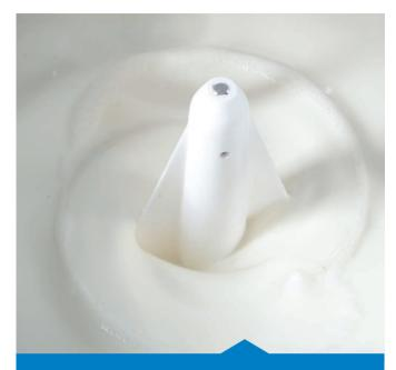
Tank agitator with adjustable speed Prevents stratification during storage and improves heat exchange during pasteurization.
